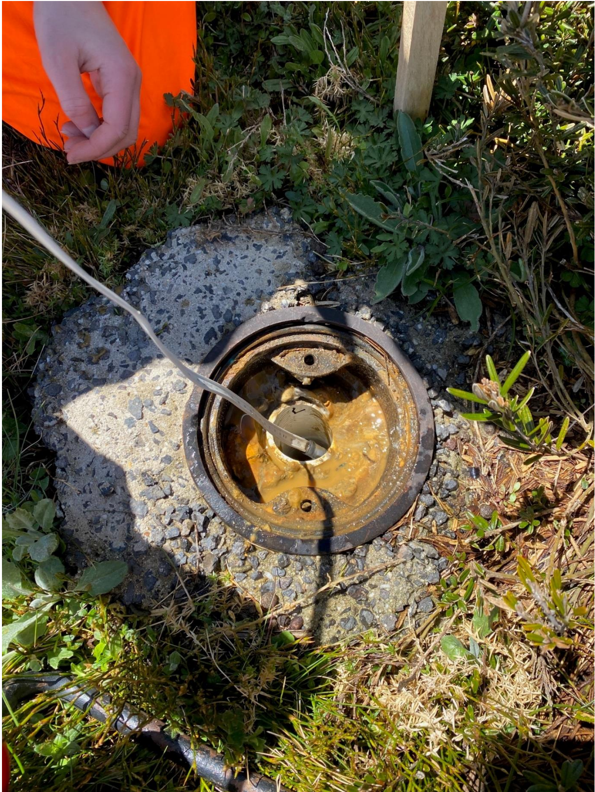
Figure 3. Example of a groundwater monitoring borehole being sampled (provided by ARV during the site meeting).
